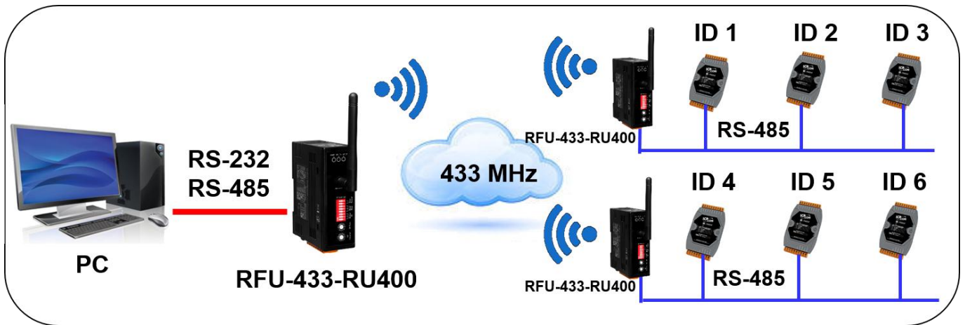
PC controls RS-485 modules 1 ~ 3 through a RFU-433-RU400 and modules 4 ~ 6 through another RFU-433-RU400
