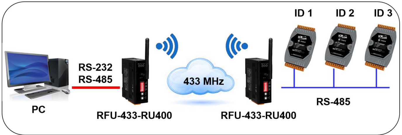
PC controls RS-485 modules 1 ~ 3 through RFU-433-RU400.
