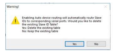
Click **Yes** to delete the existing (factory default or user-set) routing table; the auto-routing mechanism will automatically find the correct serial port that connects the target Modbus device. Moreover, if a device is added to the gateway later, the gateway can also route it correctly. Note that the routing table will be cleared as the warning message. The Slave ID table is then shown as in the figure below.
