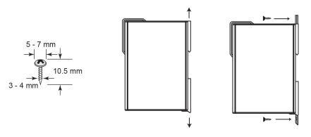
**NOTE** Wall mounting is certified for use in maritime applications. The device must be installed more than 60 cm from the compass.
