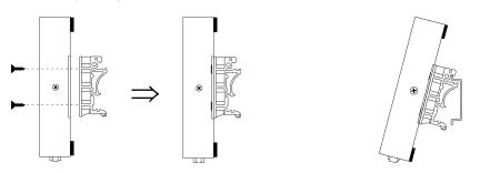
**Mounting on the wall:** You will first need to attach the mounting plates to the unit. Place four screws in the wall and slide the unit onto the screws as shown.
