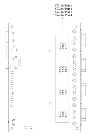
**To add a 120**  $\Omega$  **termination resistor,** set switch 3 on the port's assigned DIP switch to ON; set switch 3 to OFF (the default setting) to disable the termination resistor.
