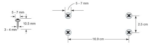
The head of the screws should be 5 to 7 mm in diameter, the shaft should be 3 to 4 mm in diameter, and the length of the screws should be at least 10.5 mm. Make sure to leave about 5 mm of space between the head and the wall.
