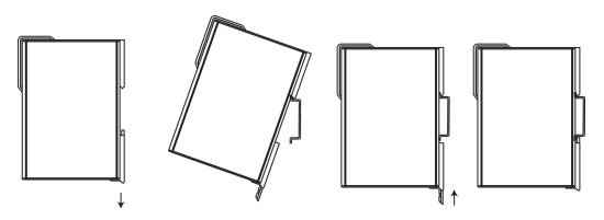
Mounting on the wall: Pull out both the top and bottom sliders and align the screws accordingly.
