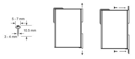
**NOTE** Wall mounting is certified for use in maritime applications. The device must be installed more than 60 cm from the compass.
