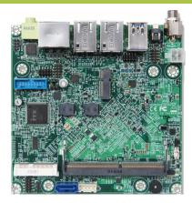
NANO-6063 is based on Intel® Atom® x6000E Series processors (formerly Elkhart Lake) integrated with Intel UHD Graphics. It supports industrial temperature range from -40°C to 85°C and can operate with TDP under 12W for fanless applications.
