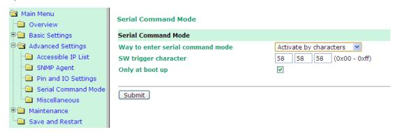
**Activate by break signal:** Break signals are caused by sending continuous Spacing values (no Start or Stop bits). When there is no electricity present on the data circuit, the line is considered to be sending a Break. The Break signal must be of duration longer than the time to send a complete byte plus Start, Stop, and Parity bits.
