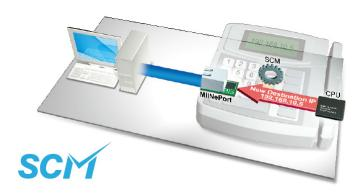
MiiNePort E1's SCM (Serial Command Mode) allows the module's parameters to be retrieved or configured through the serial port, rather than over the network. This is done using specially parsed commands sent to the module through the serial port.
