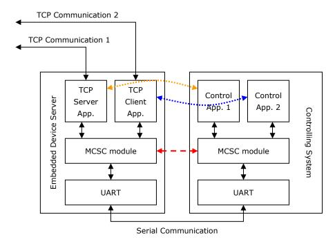
The MCSC module is built into the MiiNePort E1. To enable MCSC, you need to set your MiiNePort E1 serial port operation mode to MCSC mode and then set the channels' operation mode individually according to your application. In addition, you also need to implement the MCSC module in your device's primary system.
