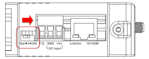
Step 2: Execute either the eSearch Utility to search for any modules connected to the network. Verify that the module has been reset to the original factory default settings. For example, the module should be shown as having the default IP address, which is 192,168,255.1.
