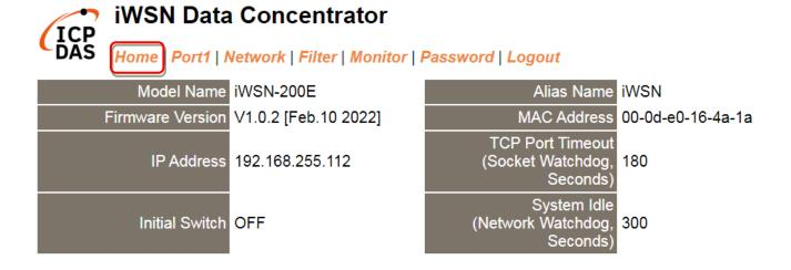
The first part of this page provides basic information about the hardware and software. The software and hardware information section includes information related to the Model Name, the IP Address, the current position of the Initial Switch, the Alias, the MAC Address, the System Timeout values, TCP Port, and the current Firmware version. If you update the firmware for the module, this page can be used to check the version information.
