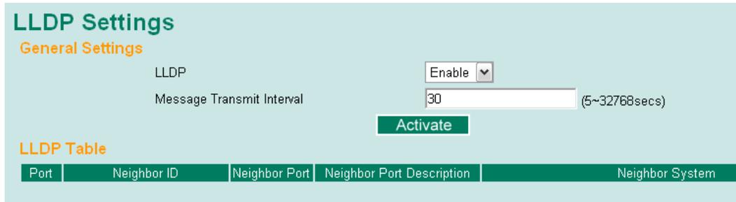
From the switch's web interface, users have the option of either enabling or disabling the LLDP, as well as setting the LLDP transmit interval (as shown in the figure above). In addition, users are able to view each switch's neighbor-list, which is reported by its network neighbors. Most importantly, enabling the LLDP function allows Moxa's MXview to automatically display the network's topology as well as system setup details such as VLAN, and Trunking for the entire network.
