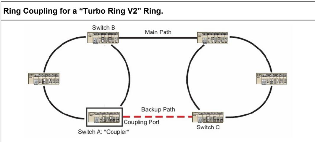
Note that the ring coupling settings for a "Turbo Ring V2" ring are different from a "Turbo Ring" ring. For Turbo Ring V2, Ring Coupling is enabled by configuring the "Coupling Port (Primary)" on Switch B, and the "Coupling Port (Backup)" on Switch A only. You do not need to set up a coupling control port, so that a "Turbo Ring V2" ring does not use a coupling control line.
