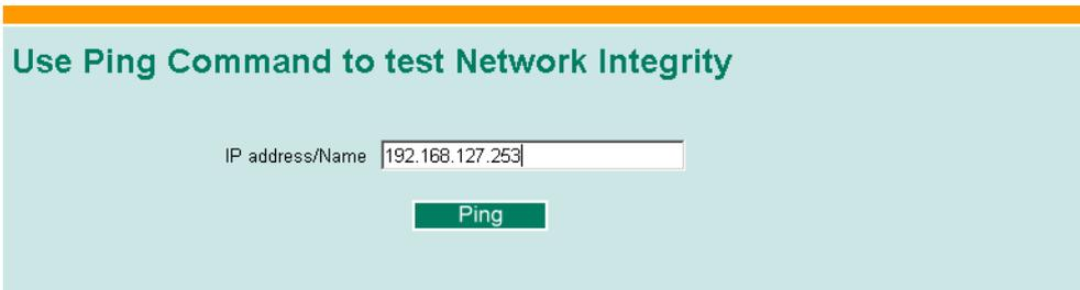
The **Ping** function uses the *ping* command to give users a simple but powerful tool for troubleshooting network problems. The function's most unique feature is that even though the ping command is entered from the user's PC keyboard, the actual ping command originates from the EDS-728 itself. In this way, the user can essentially "sit on top of the EDS-728" and send ping commands out through its ports.
