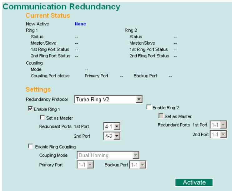
**NOTE** When using the Dual-Ring architecture, users must configure settings for both Ring 1 and Ring 2. In this case, the status of both rings will appear under “Current Status.”
