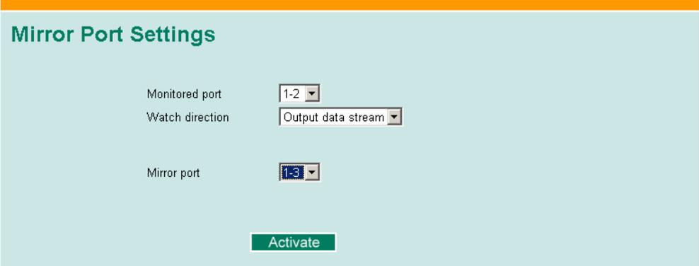
The screenshot shows the 'Mirror Port Settings' configuration interface. It includes three dropdown menus: 'Monitored port' (set to 1-2), 'Watch direction' (set to Output data stream), and 'Mirror port' (set to 1-3). An 'Activate' button is located at the bottom of the form.
