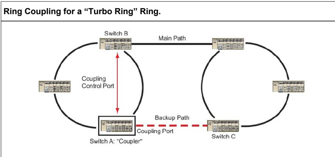
To configure the Ring Coupling function for a "Turbo Ring" ring, select two EDS-728 units (e.g., Switch A and B in the above figure) in the ring, and another two EDS-728 units in the adjacent ring (e.g., Switch C and D).
