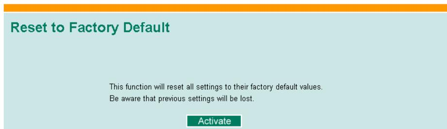
The Factory Default function is included to give users a quick way of restoring the EDS-728's configuration settings to their factory default values. This function is available in the Console utility (serial or Telnet) and Web Browser interface.
