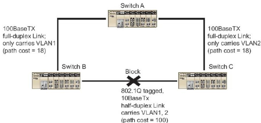
To avoid subdividing VLANs, all inter-switch connections should be made members of all available 802.1Q VLANs. This will ensure connectivity at all times. For example, the connections between Switches A and B, and between Switches A and C should be 802.1Q tagged and carrying VLANs 1 and 2 to ensure connectivity.
