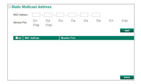
**NOTE** The MAC address (01:00:5E:XX:XX) will appear on the Static Multicast Address page. Activate IGMP Snooping to implement automatic classification.
