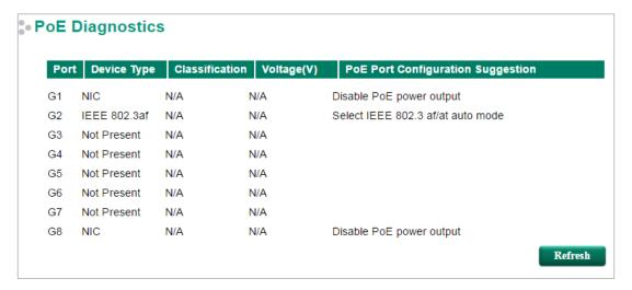
**PoE Diagnostic** helps users determine the PD conditions. The system provides the user with configuration options; select the best option for your PDs. It will automatically detect and suggest the configurations when users click on this page and the status will be refreshed when you click the refresh button.
