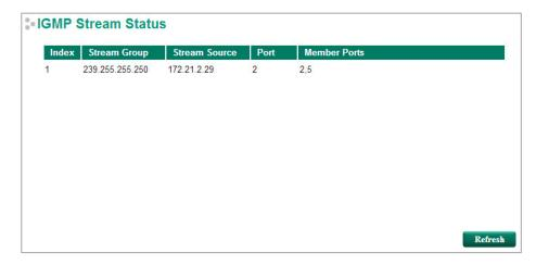
**Stream Group:** Multicast group IP address **Stream Source:** Multicast source IP address **Port:** The port that receives the multicast stream
