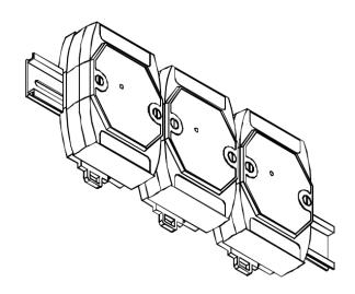
There are three new DIN rail models available. Each is made of stainless steel, which is stronger than those made of aluminum. There is a screw at one end and a ring terminal is included so that it can be easily connected to the earth ground. The three new DIN rail models are as follows.
