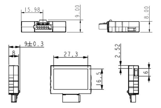
Figure 5: SATADOM D150SV-L mechanical dimensions
