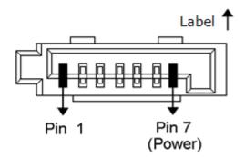
Figure 3: Signal Segment and Power Segment
