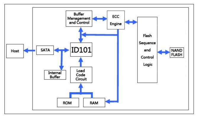
Figure 2: Innodisk SATADOM D150SV-L Block Diagram
