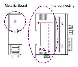
Figure 2-7 Metallic Board at Back of I-2532
