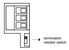
Figure 2-3 Location of Terminal Resistance Switch
