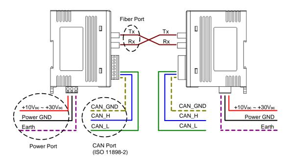
Figure 2-6 Wire Connection of I-2532
