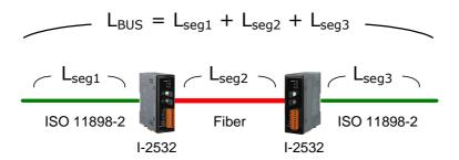
Figure 3-2 Segment Length and Bus Length
