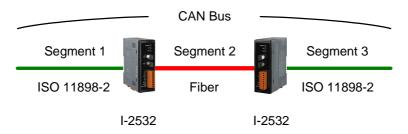
Figure 3-1 Segment in CAN bus system
