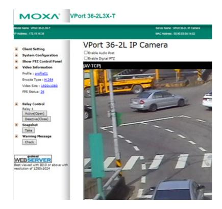
Enable the digital PTZ function by selecting the checkbox above the image view. Once the function has been enabled, you can zoom in and out on the image using the mouse wheel, and implement Pan and Tilt by pressing right button and dragging the cursor to the spot in the image you would like to focus on.
