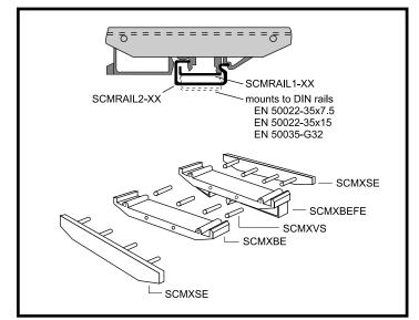
Figure 5: DIN Rail Mounting Elements
