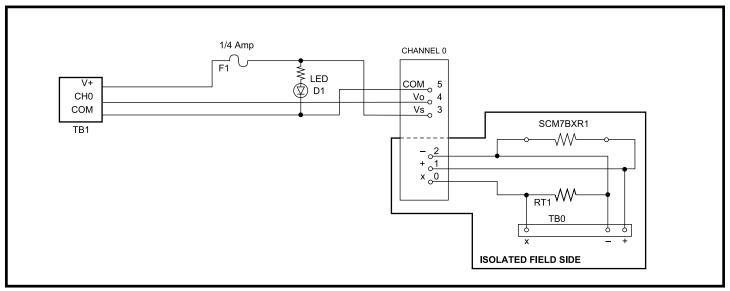
Figure 6: SCM7BP01 (-DIN) Schematic Diagram
