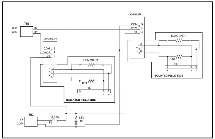
Figure 7: SCM7BP02 (-DIN) Schematic Diagram
