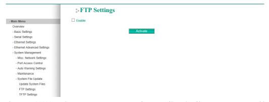
The NPort S9000 can be a FTP server to save configuration file or log files on it. You may enable it by checking the checkbox **Enable** and then click **Activate**.
