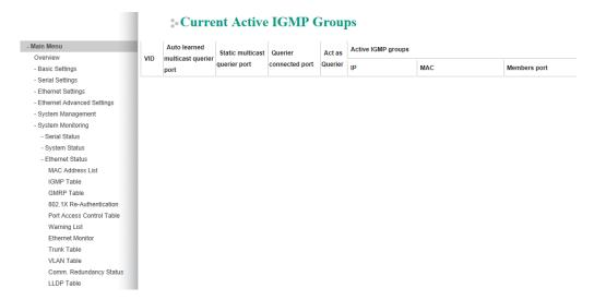
The information includes **VID**, **Auto-learned Multicast Router Port**, **Static Multicast Router Port**, **Querier Connected Port**, and the **IP** and **MAC** addresses of active IGMP groups.
