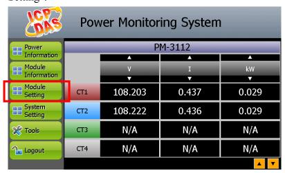
(3) Click the "I/O Interface Setting" on the "Module Setting" menu. Modify and make sure the settings of the parameters (Baudrate / Parity / Stop bits) of the COM Port that are connected to the M-7000 I/O modules are accurate. After all settings are
