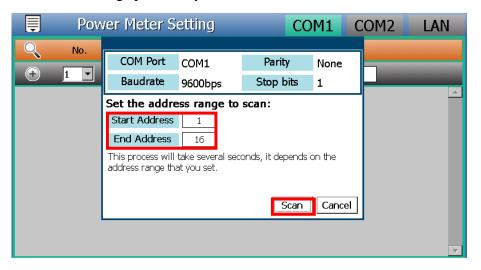
c. After the Scan operation is completed, a Modbus RTU power meter list will appear. After all settings are completed, click "Apply" button to save the changes.
