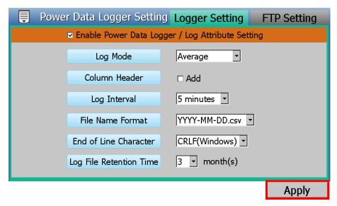
(4) If the user would like to send the power data file to the FTP server of the control center, please click the "FTP Setting" at the right-top corner of the page to enter the "FTP Setting" page.
