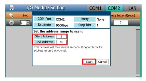
c. After the Scan operation is completed, an M-7000 I/O module list will appear. After all settings are completed, click "Apply" button to save the changes.
