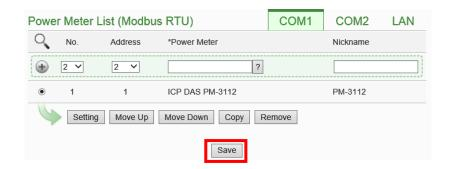
Please note: if failed to scan the power meters, please make sure the RS-485 cable is properly connected. And then go to Step 1: "System Setting"→"I/O Interface Setting" to make sure the settings of the COM Port that are connected to the power meter are accurate. After all settings are completed, click "Save" button to save the changes and repeat Step3.a to perform scanning of the power meters again.
