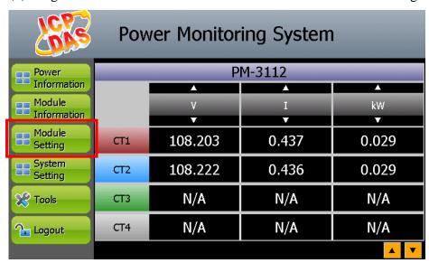
(2) Click the "Power Data Logger Setting" on the "Module Setting" menu.
