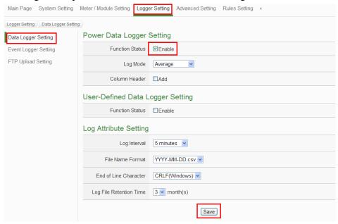
(2) If the user would like to send the power data file to the FTP server of the control center, please click "Enable" and complete settings on the "FTP Upload Setting" Page. After all settings are completed, click "Save" button to save the changes.
