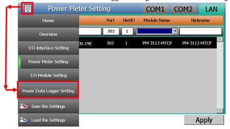
(3) Check "Enable Power Data Logger/Log Attribute Setting" to enable the Power Data Logger function. Modify and make sure the settings of the parameters. After all settings are completed, click "Apply" to save the changes.
