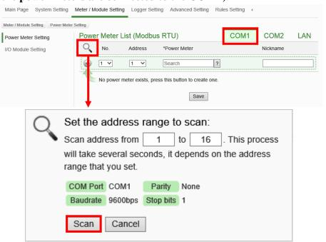
b. After the scanning is completed, the power meters connected to the COM Port interface will be displayed, click "Save" to complete the settings of the power meter list.
