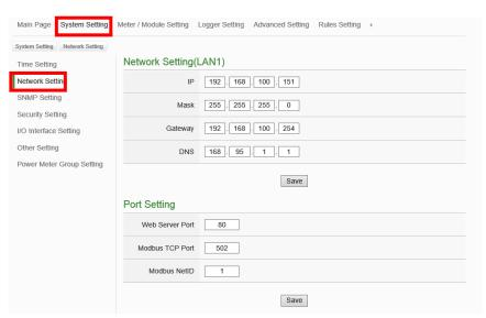
(6) After clicking on "Save" button, for the network domain of the PMD-2201 and PC are different, it is normal being not able to connect to the webpage, please connect PMD-2201 and PC to the actual network environment and then modify the network settings of PC to correct settings to connect to the PMD-2201.
