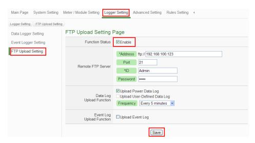
(3) Save the settings to PMD-2201, and then the Data Logger function will be enabled. The system will start to save the power data in the MicroSD card.
