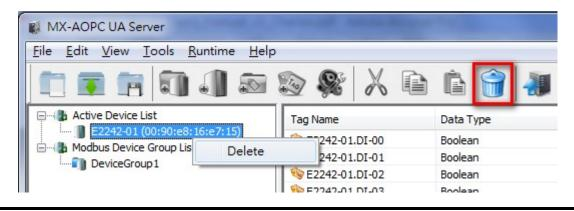
**NOTE** After an active-device name is changed through the web console or configuration utility, delete the active device on the MX-AOPC UA Server and execute "Update Configuration to Server." The change will take effect the next time the device creates active tags to the MX-AOPC UA Server.
