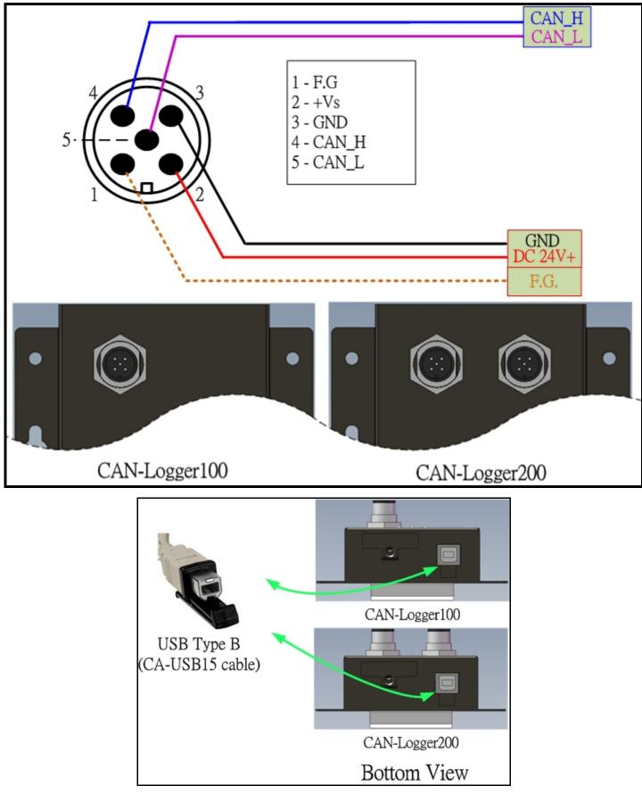
Figure 2-42 Wire Connection for CAN-Logger series
