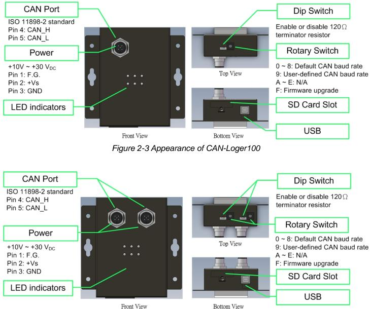
Figure 2-4 Appearance of CAN-Logger200
