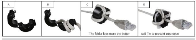
Clip-on Ferrite Core Installation
