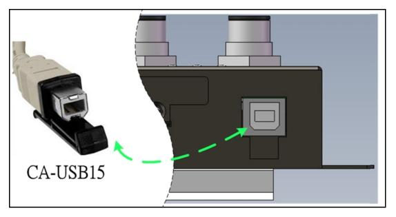
Figure 5-1 Rotary switch setting and wire connection of the USB
