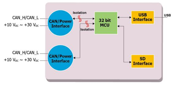
Figure 2-2 Block Diagram of CAN-Logger200
