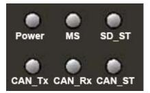
Figure 2-6 LED Assignment of CAN-Logger100
