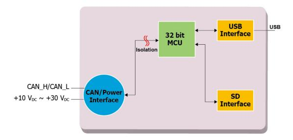
Figure 2-1 Block Diagram of CAN-Logger100
