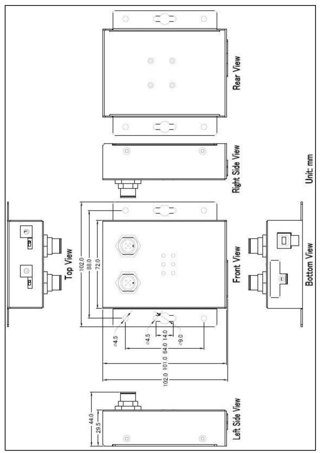
Figure 6-2 Dimension of CAN-Logger200
