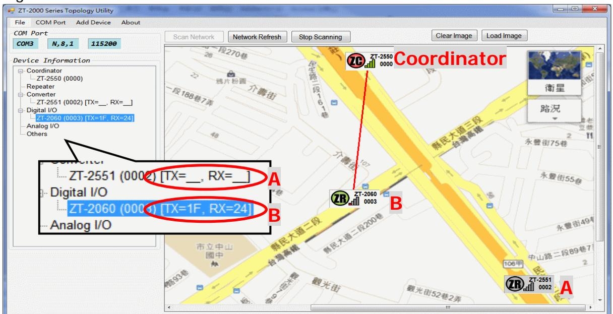
In the situation described above, the best approach is to confirm whether there is any possible interference to the signal, or if there are any obstacles affecting the network environment and, if so, add a ZigBee repeater that can be used to relay the wireless signal, as illustrated in the image below. Once installed, an improvement in the communication quality should be seen.
