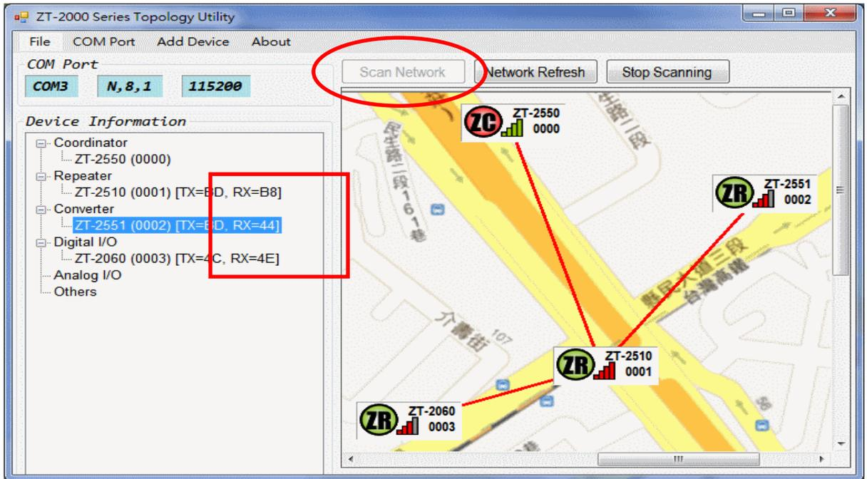
As shown in the example below, two ZigBee router devices exist in a ZigBee network. One ZigBee device "B" on the map is mounted on the opposite side to the street corner so that the signal is obstructed, which causes the signal to become weak. The other device "A" on the map is too far away, so it is unable to communicate with the ZigBee coordinator.
