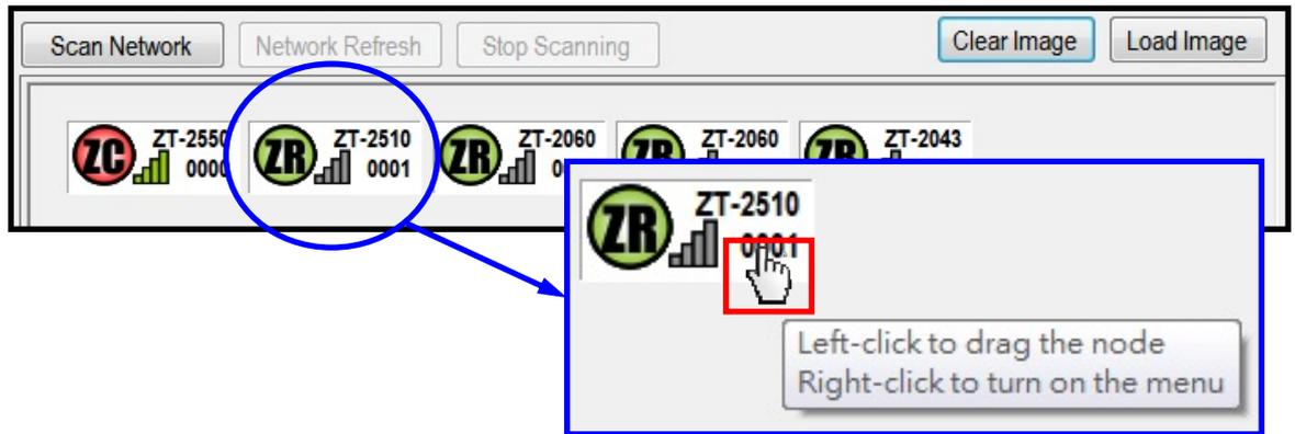
In order to view the topology of ZigBee network with the map clearly, the location of the nodes are movable. To move the position of a node, click and hold the icon for a node and then drag it to the specific location, as illustrated below.
