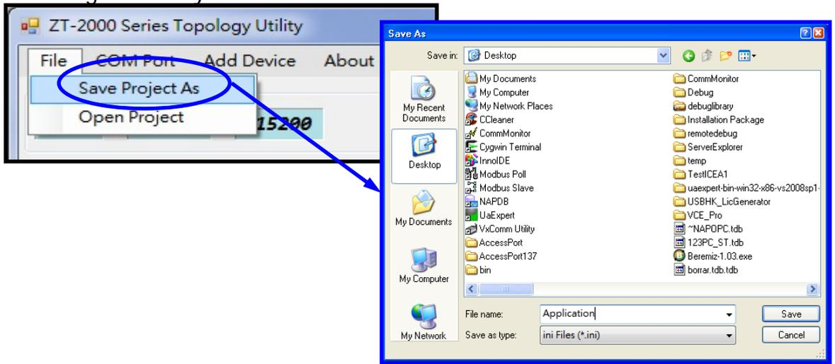
If a ZigBee network needs to be monitored again using the same settings, simply load the previously saved \*.ini file into the tool to restore the ZT-2000 Topology Tool to its earlier state, making it easy to configure the Tool for future use.
