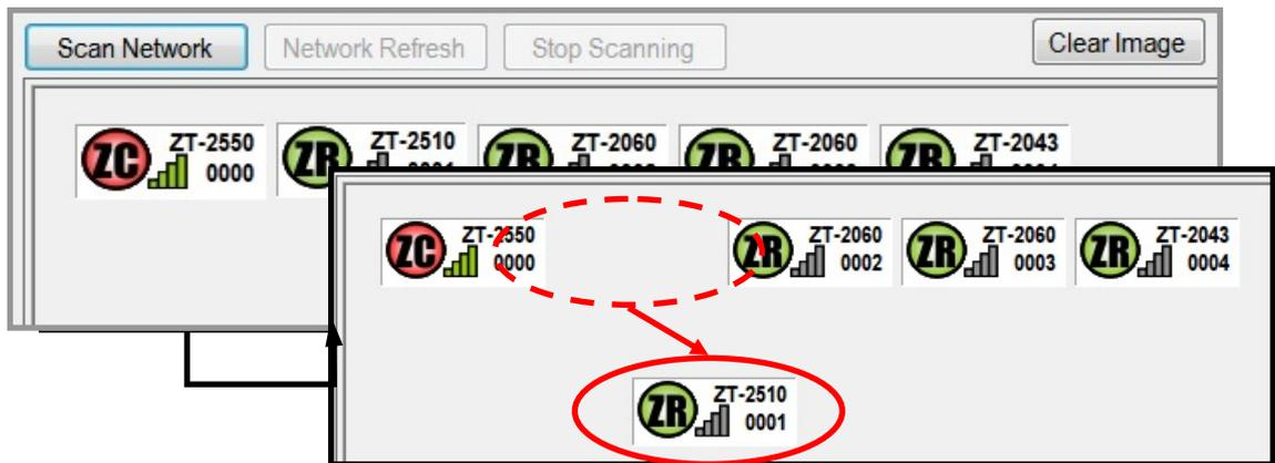
To modify the Device Information for a node, or to remove a node from the sequence, right-click the node icon and select the required option from the shortcut menu.
