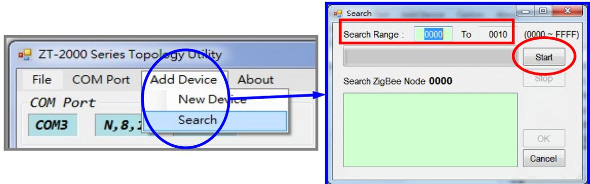
Once the search process is complete, all available ZigBee nodes will be displayed in the results field. Click the **OK** button to add the nodes to the Topology Tool for monitoring.
