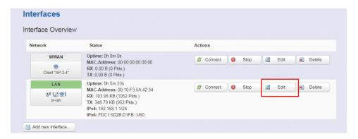
Step 2. Because LAN interface is used for device LAN connection, please make sure that Ethernet Adapter is selected in the "Physical Settings" tab.
