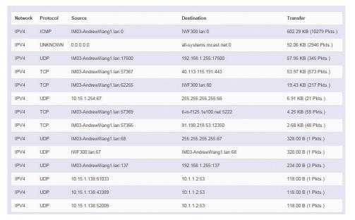
Displays NIO 51 real-time active connection information, including TCP and UDP connections.
