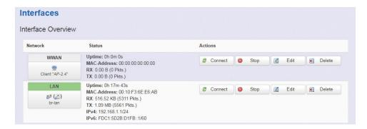
Step 2. It is suggested that DHCP client is selected if your AP has DHCP server function. Click "Switch protocol" to switch the DHCP client mode for WWAN interface.
