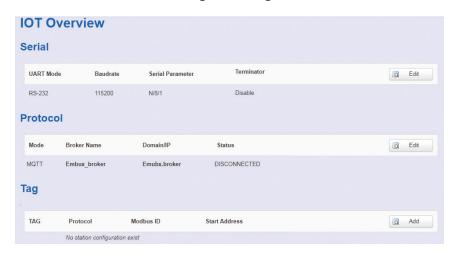
The following are Modbus parameters for configuration.
