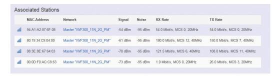
Displays current associated device information (personal computers or electronic devices) with NIO 51, including device's MAC address, signal level, noise and connecting data rate.
