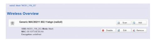
To set up the Wireless configuration, please select "Network" in the tab, then select "WiFi", which would show you the current status of radio interfaces.
