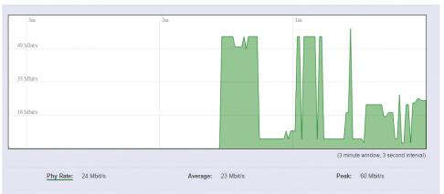
Displays wireless real-time signal quality including signal level, noise and data rate.
