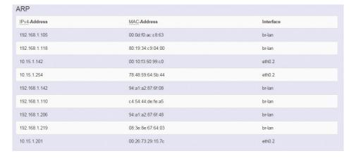
Displays ARP information in NIO 51 including IPv4 address, MAC address and connecting interface.
