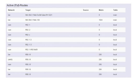
Displays active IPv6 routing table of WAN and LAN port.
