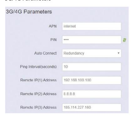
Please select "Redundancy" to enable Wi-Fi and 4G redundant function. You will then need to enter Remote IP address.
