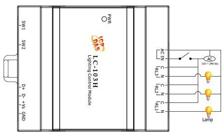
The LC-103H has a single AC input that can be used to connect a lighting control switch and three relay outputs that can be used to connect the lighting, lamp or AC LED lighting etc. Please refer to the above diagram for detailed wire connection information. The input channel of the LC-103H can directly control its 3-channel relay ON and OFF sequence without requiring a remote host controller, so it's very easy to test any lighting circuits for incomplete applications.
