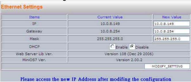
The Ethernet settings page can be used to view and change the TCP/IP network settings for the ET-6000 module.
