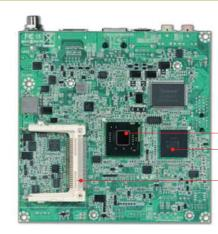
Intel® D2550 Processor Intel® NM10
