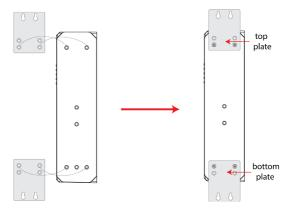
**Step 2**—Mounting the TSN-G5000 Series on the wall requires four screws. Use the switch, with wall mount plates attached, as a guide to mark the correct locations of the four screws. The heads of the screws should be less than 6 mm in diameter, and the shafts should be less than 3.5 mm in diameter, as shown in the figure at the right.
