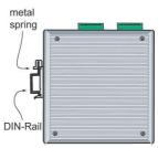
To remove the EDS-516A from the DIN-Rail, simply reverse Steps 1 and 2 above.
