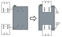
**STEP 2:** Mounting Moxa EDS-516A on the wall requires 4 screws. Use the EDS-516A, with wall mount plates attached, as a guide to mark the correct locations of the 4 screws. The heads of the screws should be less than 6.0 mm in diameter, and the shafts should be less than 3.5 mm in diameter, as shown by the figure on the right.
