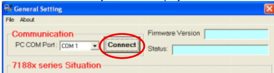
Step 6: Press the “Connect” button to connect the CANopen gateway. Then the “Com Port Scan Parameter Setting” dialog will pop up as follows. Please set the proper value for the RS-485 communication parameters. These parameters need to match with the DCON modules parameters. Then, press the “OK” button to begin the modules scans.
