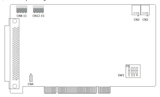
Figure 3.2 Location of Jumpers & DIP Switch
