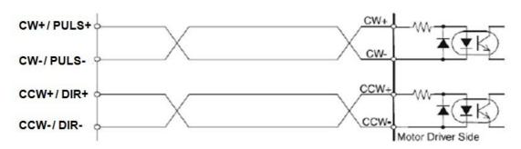
Figure 3.4 Photocoupler Interface
