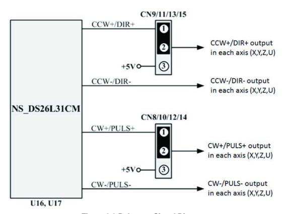
Figure 3.3 Pulse out Signal Diagram
