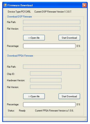
The tool is to upgrade the FPGA firmware. There is no DSP firmware download function in PCI-1245L. Both download and upgrade procedure are the same, but you shall be aware that the PC is necessary to reboot after FPGA firmware upgraded. Then, the new FPGA firmware will be truly updated.
