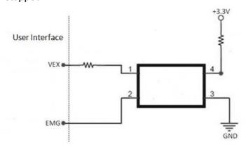
Figure 3.8 Circuit Diagram of Emergency Stop Input Signal
