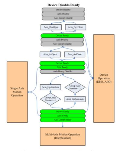
**Figure 6.2 Basic Operation Flow Chart**
