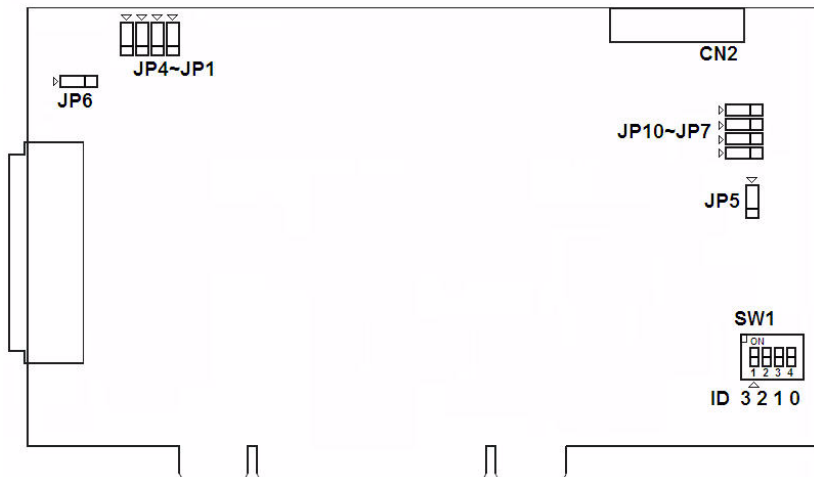
Figure 3.2: Location of Jumpers & DIP Switch
