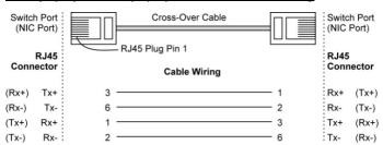
**NOTE** If the PD only supports MDI mode (V+, V+, V-, V- for pins 1, 2, 3, 6), choose a cross-over Ethernet cable to connect the PD and the EDS switch. If the PD only supports MDI-X mode (V-, V-, V+, V+ for pins 1, 2, 3, 6), choose a straight-through Ethernet cable between the PD and the EDS-P206-4PoE switch.
