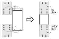
**STEP 2:** Mounting the EDS-P206A-4PoE on the wall requires 4 screws. Use the switch, with wall mount plates attached, as a guide to mark the correct locations of the 4 screws. The heads of the screws should be less than 6.0 mm in diameter, and the shafts should be less than 3.5 mm in diameter, as shown in the figure at the right.
