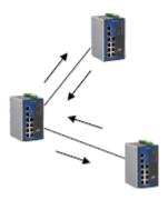
From the PRP/HSR RedBox's web interface, you can enable or disable LLDP, and set the LLDP transmit interval. In addition, you can view each PRP/HSR RedBox's neighbor-list, which is reported by its network neighbors. Most importantly, enabling the LLDP function allows Moxa's MXview to automatically display the network's topology and system setup details, such as VLAN and Trunking, for the entire network.
