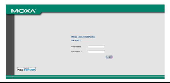
**NOTE** By default, the password assigned to the Moxa PRP/HSR RedBox is **moxa**. Be sure to change the default password after your first log in to maintain a higher level of security.
