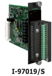
8-channel Thermocouple Input Module, Include CN-1824M
