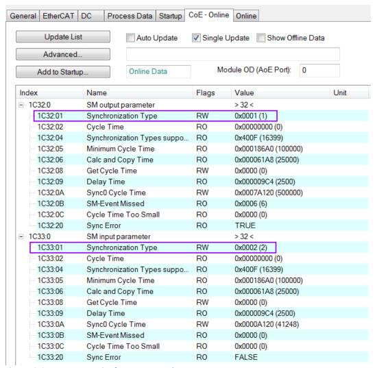
Figure 16: SyncManager setting for Free-Run mode
