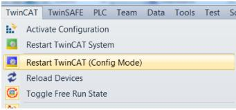
Figure 26: Download PDO assignment and restart TwinCAT
