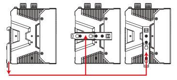
**STEP 2—**Insert the upper lip of the DIN-rail kit into the mounting rail.
